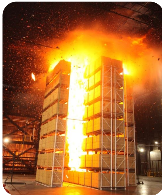
Ceiling-Only Sprinkler Inadequate 仅用顶棚喷淋的不足
